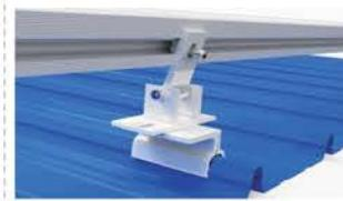
**Step2.** Insert the nut of tilt leg into the rail channel, and fasten the bolt and nut to fix the rail.
